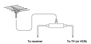
Connecting the antenna cable to the 75/300  $\Omega$  antenna adapter (For all models other than USA & Canadian models and European models)
